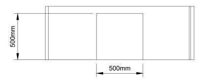
Place a slab or similar hard standing base into the bottom of the excavated hole. Ensure this is level
