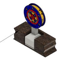
Within the allocated space excavate 500mm x 500mm x 450mm.
