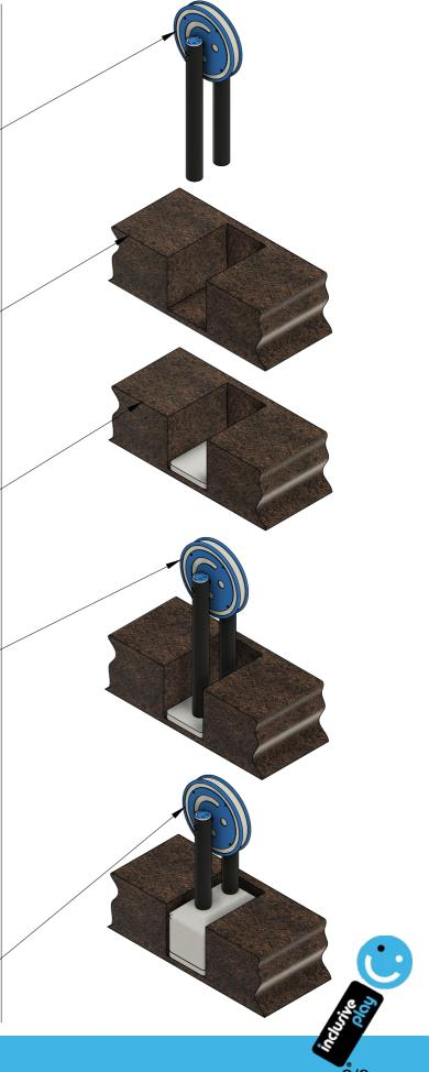
Within the allocated space excavate 400mm x 610mm x 450mm.
