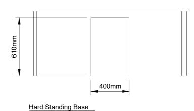
Place a slab or similar hard standing base into the bottom of the excavated hole. Ensure this is level.
